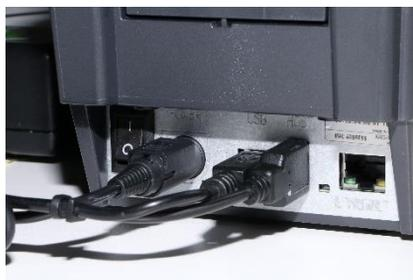
3. Connect the DC powerpac to the printer and to mains power then turn on the power. Once booted up press the ESC key to confirm the software version on the top line. This should match the reference chart supplied
