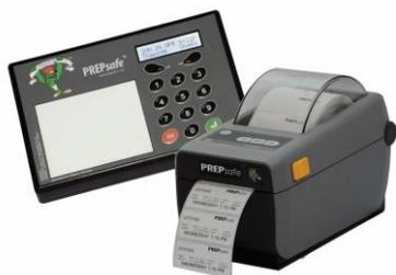
2. Connect both USB cables from the PREPPY console to the printer. Each plug is different so therefore can only be connected one way
