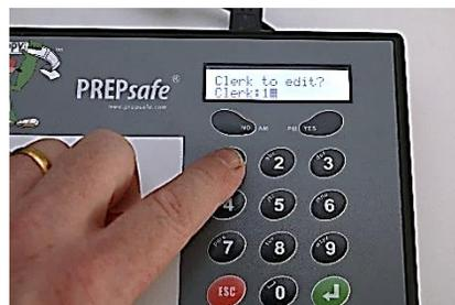
6. Use the same managers menu to adjust both date and time, note when setting am/pm the corresponding buttons are the same keys as yes/no
