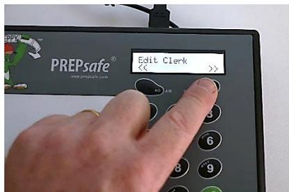
5. Select a clerk number to edit (between 1 – 99) press enter then using the SMS keypad enter the clerk name and then press enter to confirm
