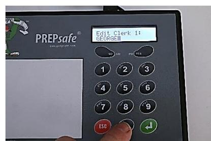
7. To Print a label press the top right key “Use-By” then enter the corresponding Item number from your reference chart and press the enter key
